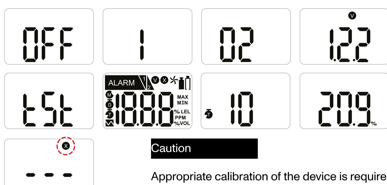
Appropriate calibration of the device is required prior to operation. Always ensure that the device responds correctly to the relevant gas. Verify that foreign materials that could interfere with the detection of gas are not blocking the sensor.
