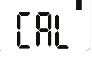
Once completed, will appear for several seconds on the display. The device will then return to Gas Measurement mode.
