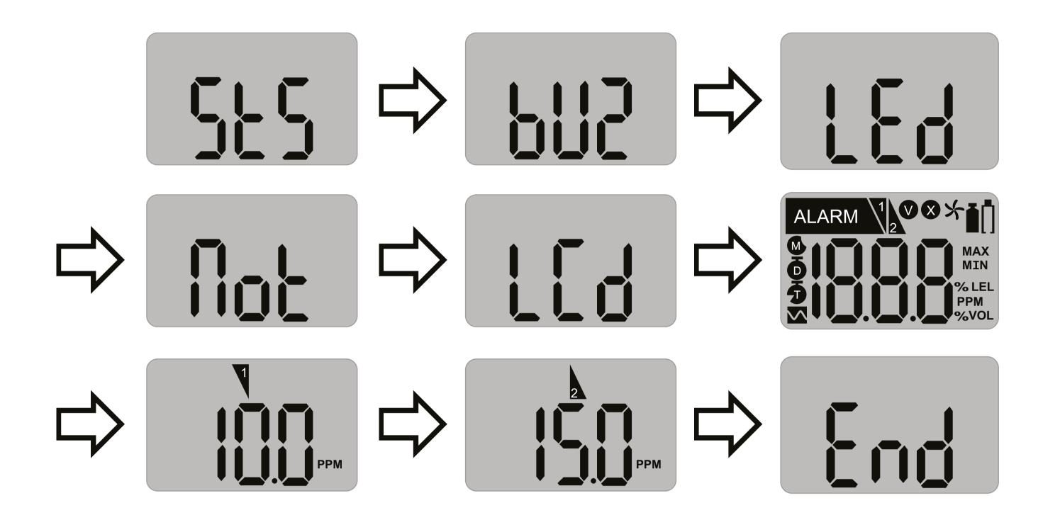
Press the button to initiate the Self Test function.
