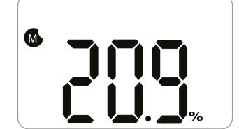
Following activation the device will operate in Gas Measurement Mode. The remaining sensor life (default setting) or gas concentration (configurable option) will be displayed on the screen. Oxygen concentration is displayed in percent by volume (%Vol) and toxic concentration is displayed in parts per million (PPM).
